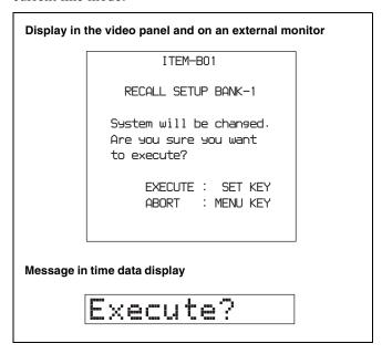
Press the SET button to recall the settings and switch to the line mode saved in the menu bank. When you power the unit off and then on again, it will use the line mode and settings of the selected bank.
